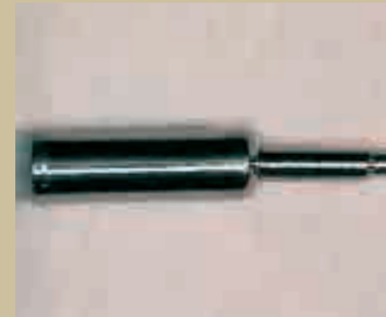
冷陰極蛍光管電極溶接 CCFL Welding
